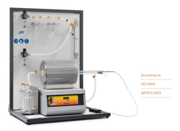
Statutory standards prescribe the verification of carbon black content of polyolefin plastics. The test method is based on pyrolitic decomposition of the material in an inert gas flow (nitrogen). This means that the remaining quantity is burned once again under forced ventilation at the same temperature and the carbon black content determined by means of weight difference.
